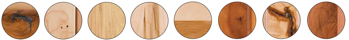
Open knot Worm holes Worm tracking Mineral streaks Vibrant color Closed knot Bark pockets Non-structural splits
